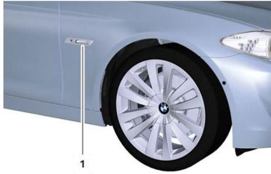
1 Parking assistant ultrasonic sensor in the side marker turn signal indicator
