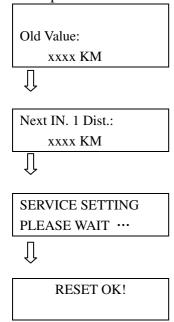
To Reset Inspection I Time use channel To:12.
